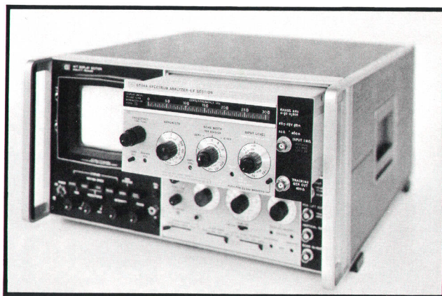
Fig. 1. A new plug-in LF Section for the HP Spectrum Analyzer family to 300 kHz, features built-in tracking generator and crystal markers. A low-noise isolated front end provides high sensitivity (20 nanovolts) and freedom from ground-loop pickup. Absolute calibration in power for several impedances is provided, with an option for balanced input.
